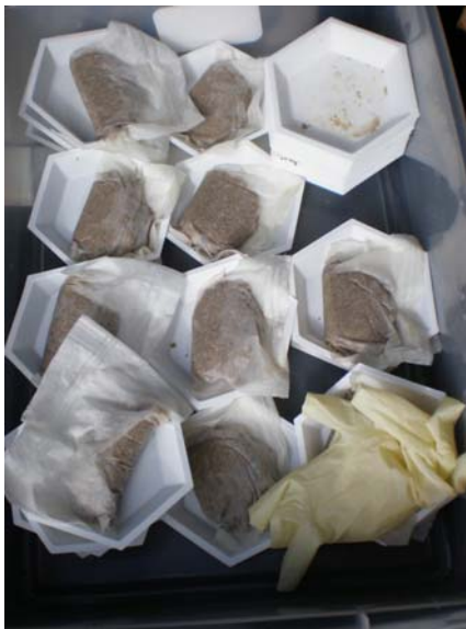
Figure 1. Porous sand bags inoculated with three marked strains of generic E.coli . Method used as field inoculum for practice effectiveness monitoring.
