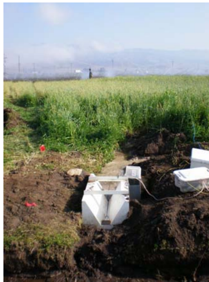
Figure 2. Illustration of flume with automatic water sampler used during grassed waterways and polyacrylamide field trials.
